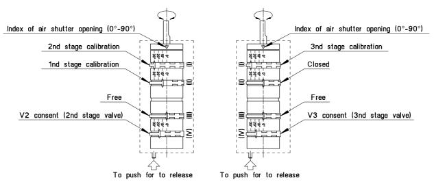
AIR SERVOMOTOR  $1^{\circ}-2^{\circ}$  ST. LANDIS
